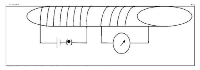
(ii) When key is closed, there is deflection in galvanometer.
